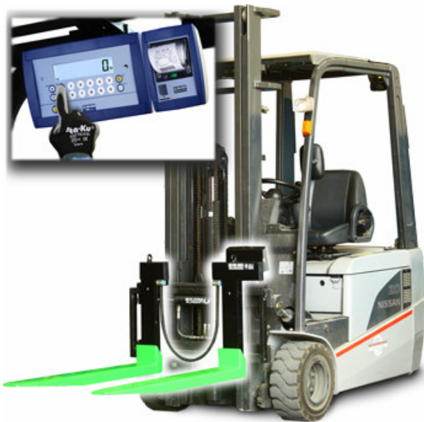
LTF09: pair of weighing forks. Indicator for mounting in the cabin, with optional printer.
